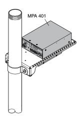
Attach input and output cables to the mounted device and thread them through the access hole in the projector pipe to the inputs and the display device. Use the remaining tie wraps for cable tidying.
